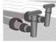
Low Point Drains
