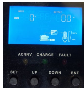
Press the DOWN button twice to get to the PV Screen from Main Screen
