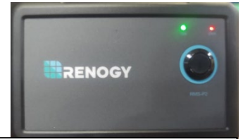
Inverter Charger On/Off Remote Red Light = Inverter Fault
