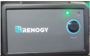
Inverter Charger On/Off Remote Green Light = Inverter Powered
